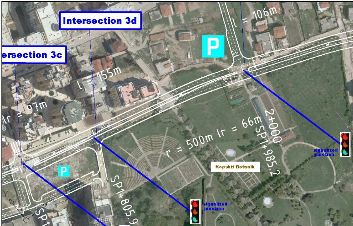
Figure 6: Crossing the Botanic garden (km 1,805-1,985)
