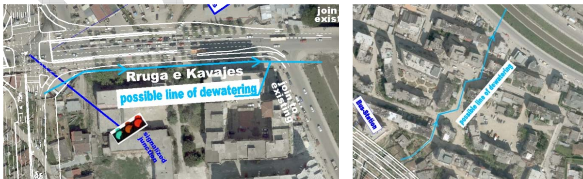
Figure 16: Dewatering concept – km 0,0+00 – 2,9+00
